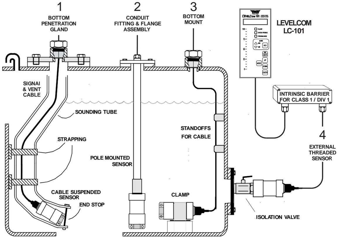
Figure 8 In Tank Sensor Mounting Options
