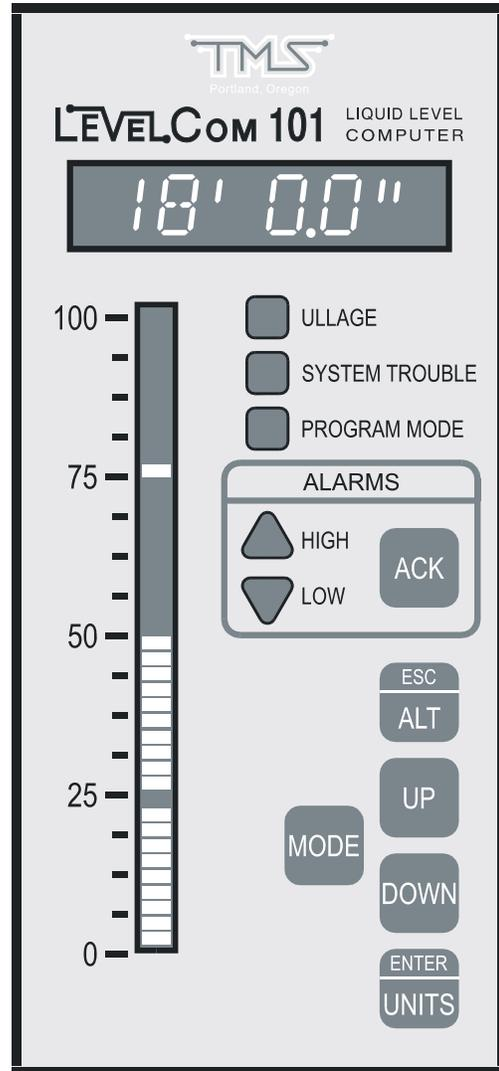
**Figure 2 Display With Visible Alarm Setpoints**
