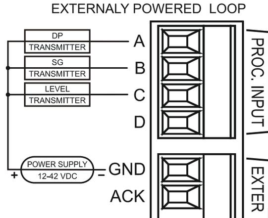
**Figure 12 Externally Powered Sensor**
