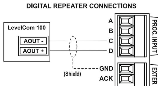
**Figure 13 Digital Repeater Wiring**
