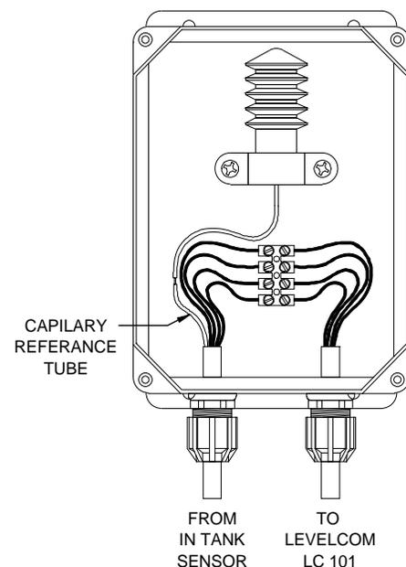
**Figure 10 Bellows Mounting**
